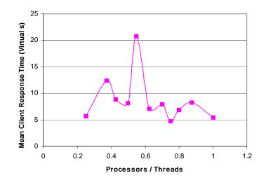
Figure 7.3: Client response times for different number of threads, processors = 40
